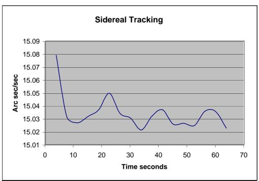
This graph is of the raw Sidereal tracking rate of a LX200GPS. The scope is in polar mode and PEC & Smart Mount are turned off
